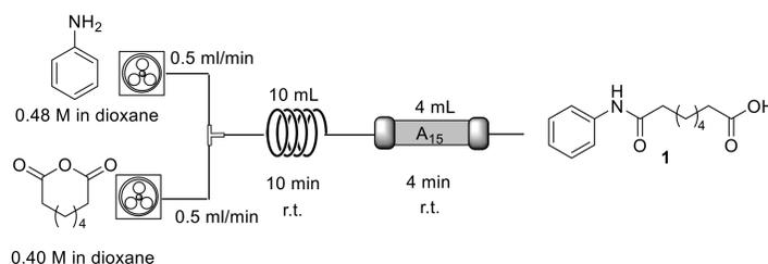
The resulting crude, in which suberanoyl acid and the excess of aniline were present, was then purified in-line passing through a glass column reactor packed with acidic resin **Amberlyst® 15 to catch the aromatic amine and readily protonate the desired carboxylic acid**. Pure **compound 1** was collected after the removal of the solvent under reduced pressure.
