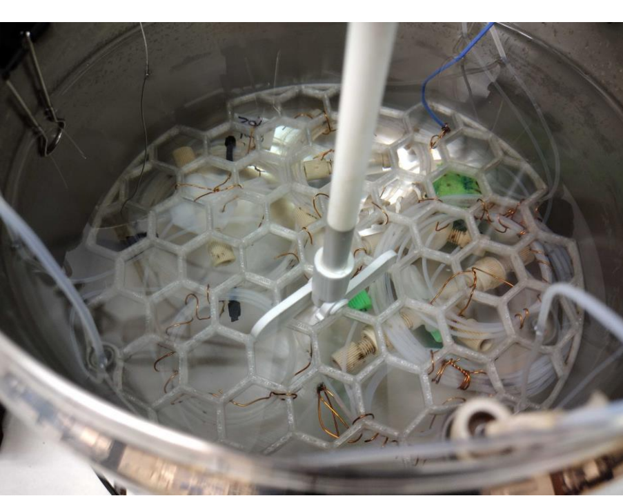
Cooling bath (jacketed beaker) with 3D printed holder for reactors G1, R1, R2 and L1-L5; efficient mechanical mixing
