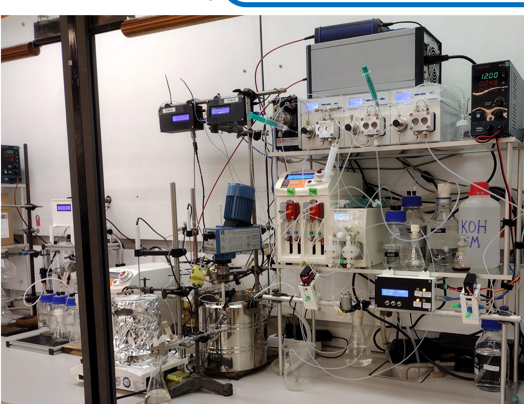
Overview of the continuous flow nitration setup: pumps, automated valves, metal jacketed beaker (cooling of reactors G1, R1, R2), p/T readers visible; FSM is on the left side
