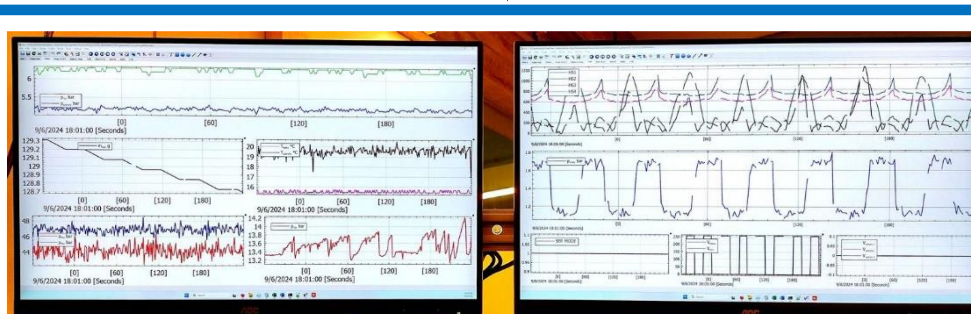
Screens for plotting real-time process parameters, e.g. pressure, temperature, HNO 3 pumping, state of the FSM; Data acquisition custom software created in Python
