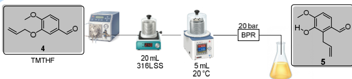
Scheme 2. Claisen rearrangement in TMTHF under flow.
